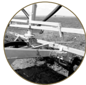
Elevator system can be raised up to 3 meter height to ease irrigating long height crops
